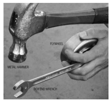
**REMOVING THE NUT WITHOUT AN AIR WRENCH**
